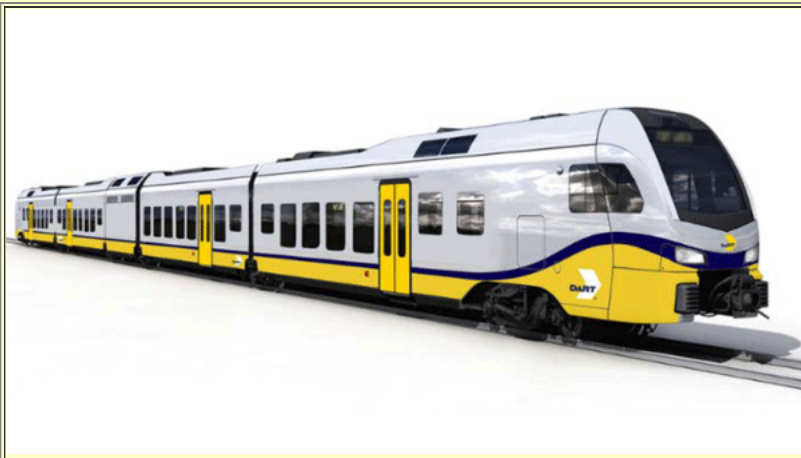
Stadler Concept DART Five Unit Diesel Multiple Unit (DMU) train.
